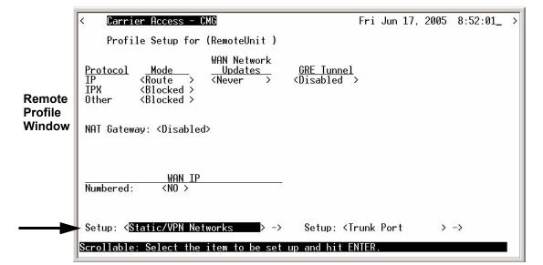
4. Select [CTRL A] to add a Static IP Network. Enter Network Address, Subnet Mask and Metric value.
